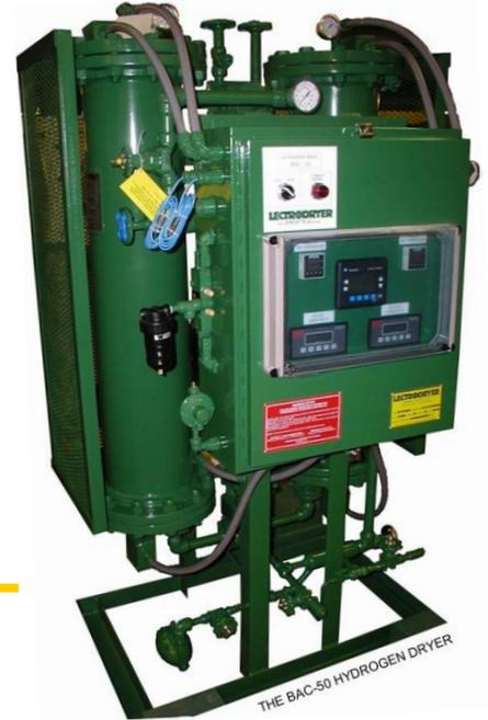
Interlocked non-lubricated 4-way valves provide trouble-free switching with a generously sized double acting actuator. Reactivation is accomplished at operating pressure with a closed circuit system with **no hydrogen purge loss** or Infiltration of air into the system.
