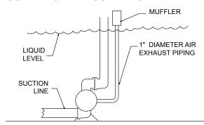
Pump can be submerged if the pump materials of construction are compatible with the liquid being pumped. The gas exhaust must be piped above the liquid level. When the pumped product source is at a higher level than the pump (flooded suction condition), pipe the exhaust higher than the product source to prevent siphoning spills.
