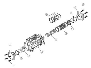
**Valve Assembly for Aluminum Mid Sections**
