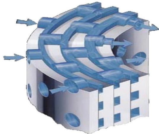
Similarly, for noisy applications, the focus of the solution to the unwanted noise originating in the valve is through use low-recovery trim packages that break up the flow into smaller flows, as well as multi-stage pressure reducing cylinders.
