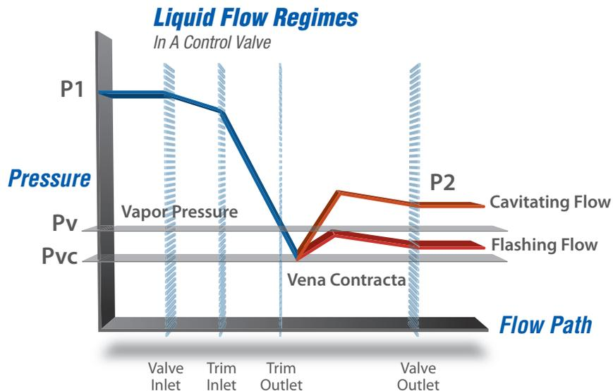
Both cavitation and flashing tend to cause hydrodynamic noise in a valve, but aerodynamic noise in gas or vapor service is typically what constitutes a noisy problem valve. Aerodynamic noise in valves is caused by fluid turbulence that typically originates within the valve body. First, fluid turbulence, and thus noise, can occur within
