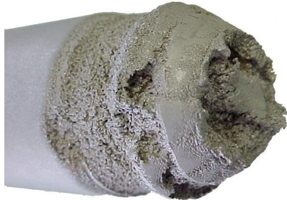
Control Valve Plug Damaged by Cavitation
