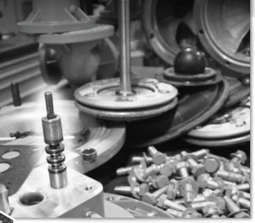
The Air Motor's Pilot Valve is the Most Often Serviced Part on an AODD Pump
