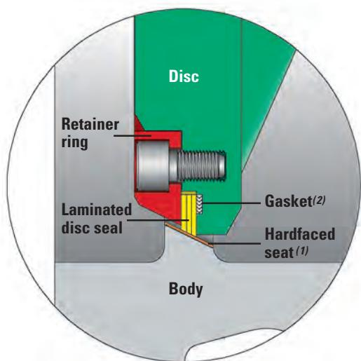
Velan provides an extra rigid retaining ring with bolting, designed in response to ASME stress calculations.
