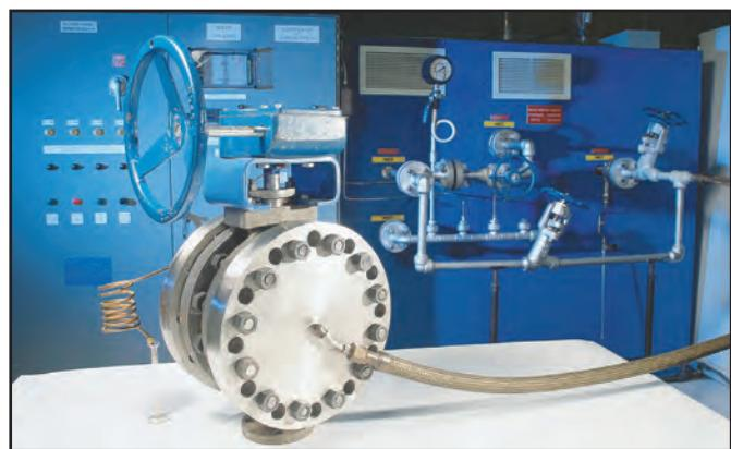
Superheated test on NPS 14 (DN 350) class 150 valve.
