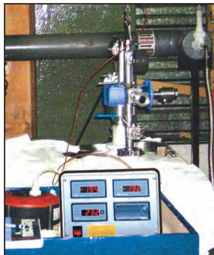
Cold temperature testing to -314°F (-192°C) of the cryogenic Torqseal® valve in our Lyon, France facility.
