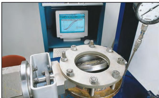
NPS 8 (DN 200) class 150 valve, ambient cycling.
