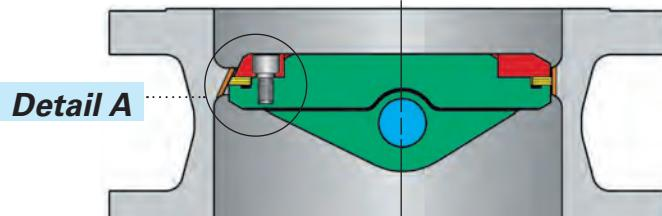
Raised, conical seat prevents solids build-up from interfering with the seal. Seat is hardfaced with CoCr alloy to meet severe service (in lieu of soft 316SS hardfacing).
