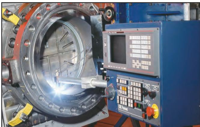
Automated CoCr alloy (cobalt-chrome alloy) deposit system.
