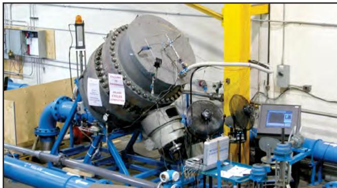
Velan Torqseal® valve with renewable seat ring and Ti O<sub>2</sub> plasma sprayed seat surface.
