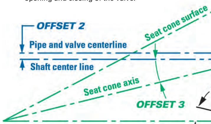
**OFFSET 3:** The seat cone axis is offset from the shaft centerline to eliminate friction during closing and opening and to achieve uniform compressive sealing around the entire seat.
