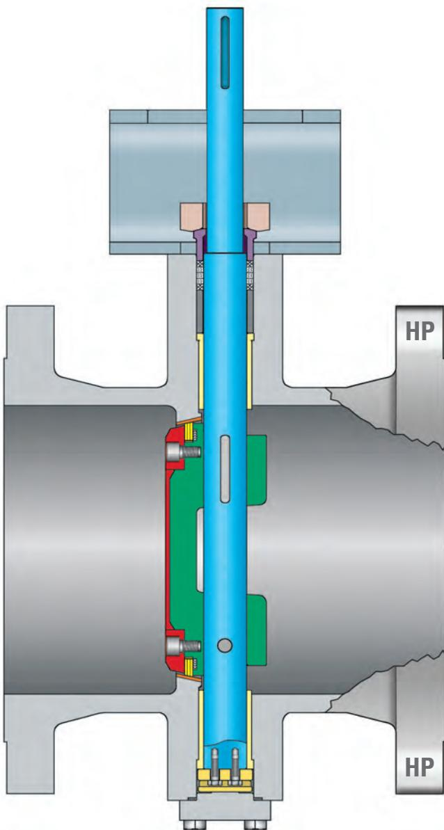
**NOTE:** The valve is marked HP for the preferred pressure side when installing the valve (shaft side is the high pressure side for flow assisted sealing). Valve is bi-directional.
