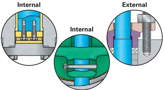
The Torqseal® advanced design features three-way eccentricity and unique elliptical seat geometry ensuring compressive sealing around the entire seat and a tight, bubble free valve.
